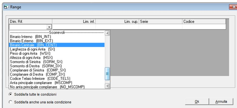
**Internal track (BIN\_INT):** applies the fitting if the panel that FP\_PRO is analysing is movable and is located on the internal track (e.g. drip channels).
