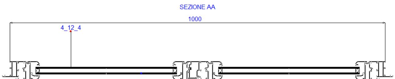
The section can be dimensioned exactly as explained in the previous paragraph. The purpose of this function is that it allows sections to be exported to a CAD program in a scale of 1:1.
