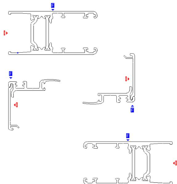
The multi-joint positions itself normally without the need to turn over any of the profiles.
