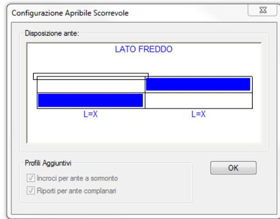
This is very useful in multi-joint composition as it helps distinguish the internal track from the external.
