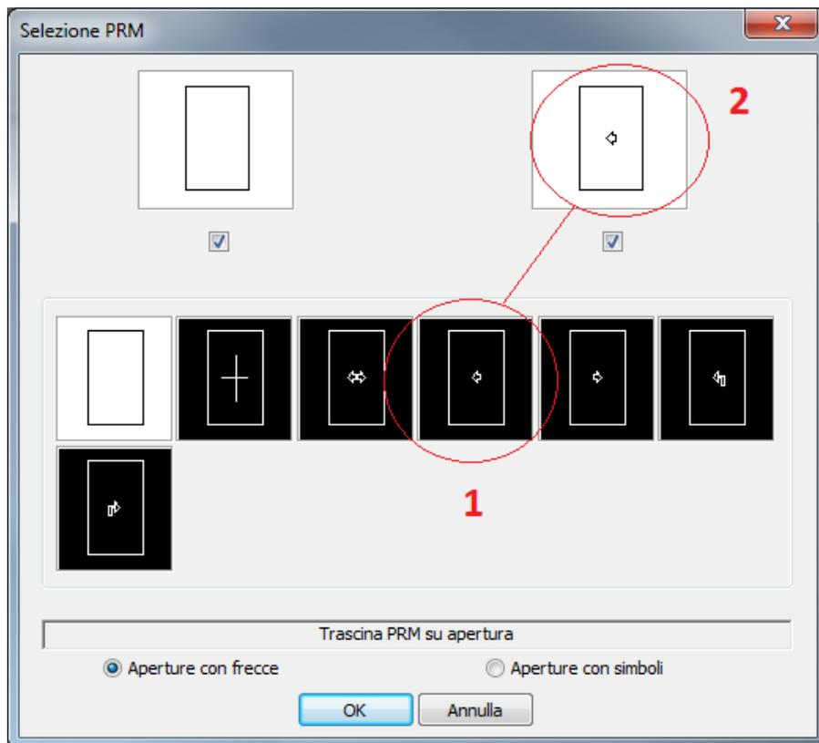
The two rectangles at the top of the screen represent the panels of the sliding system. To associate the opening type image with each panel, simply position the cursor on the PRM and, using the mouse, drag and drop it on the relative panel.
