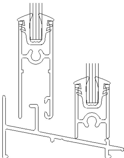
The use of a lower inclined frame that requires 2 vertical panels of different sizes
